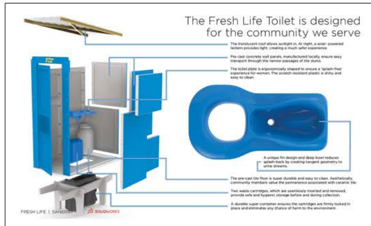
In Kenya, Sanergy's "Fresh Life" toilets use a urine-diverting squat plate
