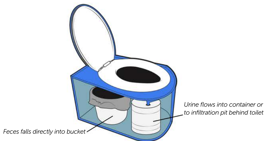
In Kenya, Sanivation uses the "Blue Box" toilet
