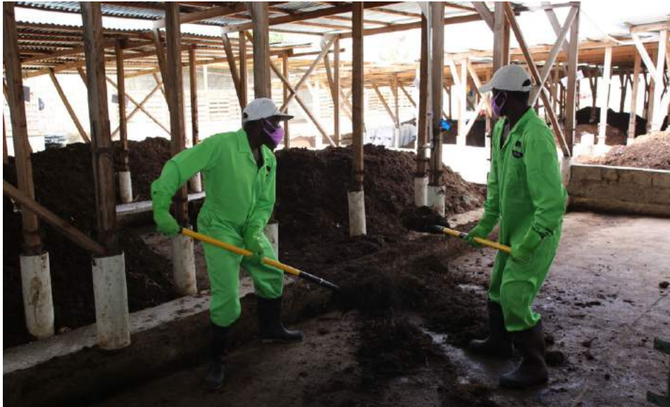
Figure 21: turning a pile of waste to increase decomposing rate
