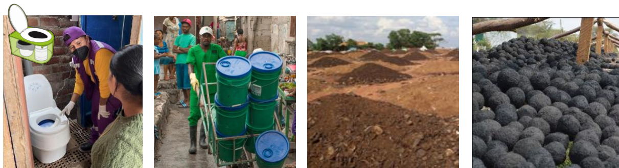
Examples of the CBS chain, including: a Sanima toilet, container collection by SOIL, composting of waste collected by Clean Team and briquettes made by Sanivation.
